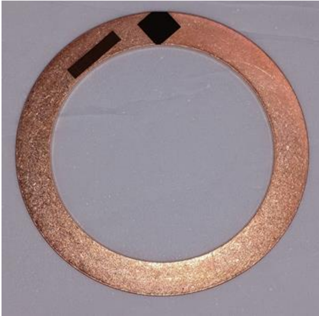
Figure 4-9: Nd:Vanadate, (Nd:YVO 4 ), laser machining of Faraday Cup array. Laser machining was performed on OFHC copper gasket to mill an array of micro Faraday Cups to act as a secondary electron suppressor. The dark rectangle seen at the top of the gasket was milled in a cross hatch pattern with an average laser power of 3 watts.
