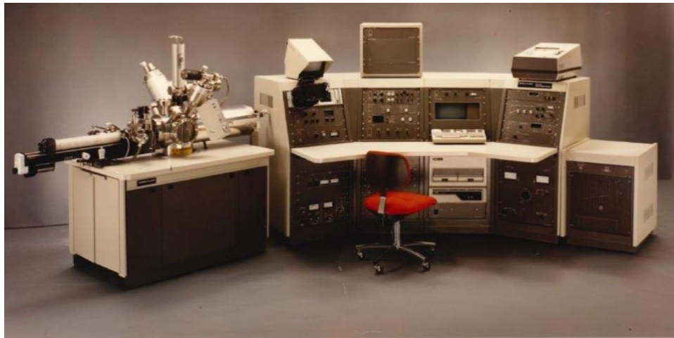
Figure 1-1: A vintage full size commercial electron spectroscopy system, [Authors photograph].
